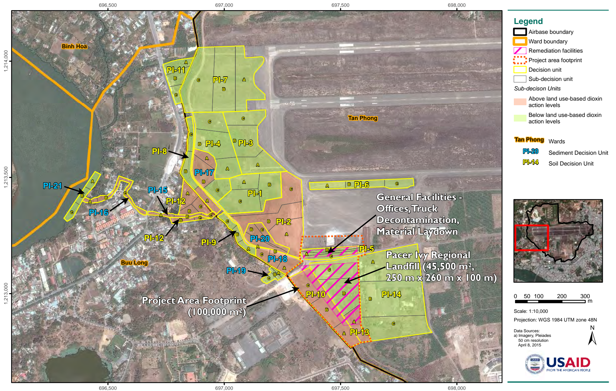
FIGURE 4-3 CONCEPTUAL LAYOUT OF ALTERNATIVE 2A IN THE PACER IVY AREA, BIEN HOA AIRBASE, VIETNAM
